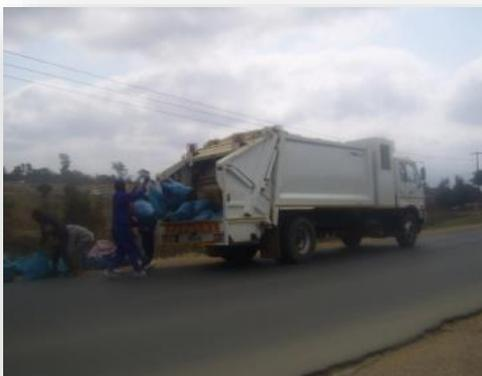
**Figure 16 : 11m3 Refuse Compactor Truck stationed at Dzanani Region**
