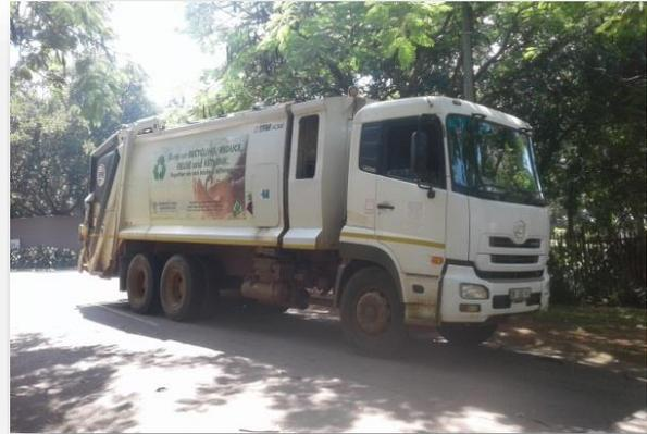
**Figure 19: 22m3 Refuse Compactor truck stationed at Makhado Region**
