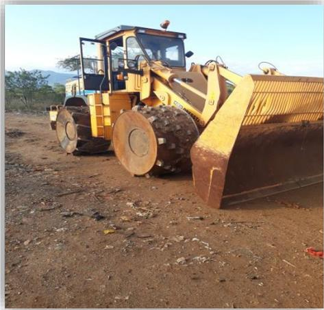
**Figure 14 : Dressta Landfill Compactor Machine**
