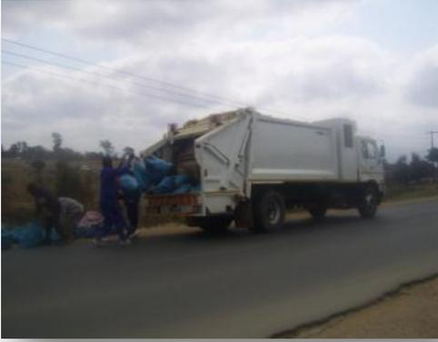
**Figure 14 : 11m3 Refuse Compactor Truck stationed at Dzanani Region**
